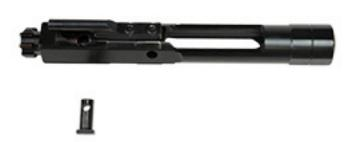
10. Remove the cam pin by lifting it out and away from the bolt and bolt carrier.
