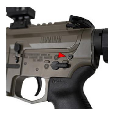
Pivot the lower receiver down and away from the upper receiver.
