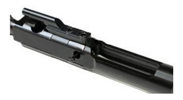
7. Push in the firing pin retaining in from right to left of the bolt carrier group and remove the pin by pulling it out to the left.
